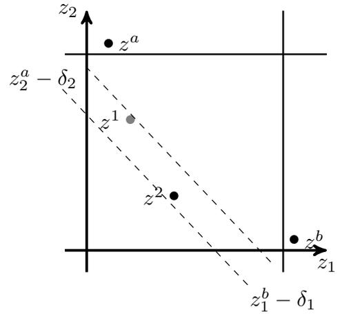
(b) Dashed lines are level lines of the objective function. Non-dominated point  $z^2$  is discovered.
