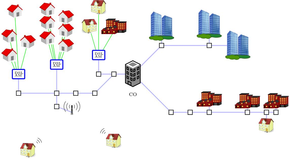
Figure 3: Schematic view of an access network using different technologies (fiber, copper, and wireless); cf. (25)
